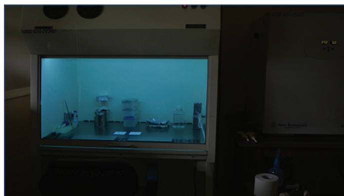
[Table/Fig-5]: Resin cements sterilisation by using Ultraviolet (UV) light for 20 minutes.
