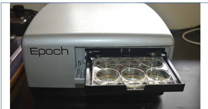
[Table/Fig-7]: Epoch Microplate Reader (Biotek Instruments, highland Park, VT,USA). (MTT (3-(4, 5-dimethylthiazol-2-yl)-2, 5-diphenyl tetrazolium bromide) assay). SoloCem (Coltene/Whalident AG,Switzerland) as group 1 and SMART CEM 2 (DENTSPLY, USA) as group 2 and control group as group 3 were evaluated.
